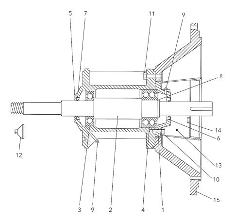
SAE power frame for models 3756 mechanical seal and packed box pumps
